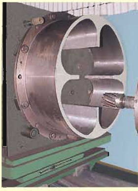
Machining of 6.5MW DCB Coupling, outer member 1.2 metre in dia
